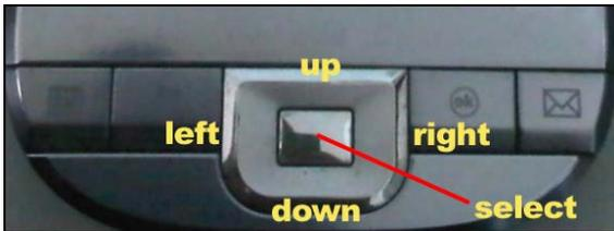
On the main screen, the up/down buttons will advance through the GunList, loading the next gun on the list into the work area. The right/left buttons will switch the display through the 4 targets.
