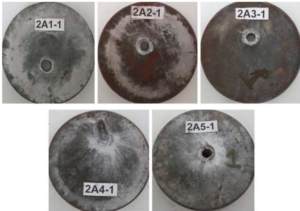
Figure 6.2: Post mortem images of HRC 39.5 samples from the 1st to 5th areal density respectively (front faces)
