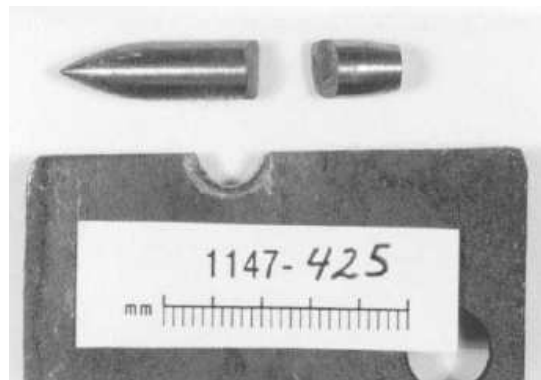
Figure 1.5: Photograph of fractured core due to edge effect [11]
