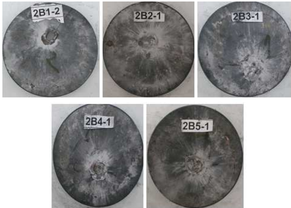
Figure 6.4: Post mortem images of the front faces of HRC 49.5 samples from the 1st to 5th areal density respectively
