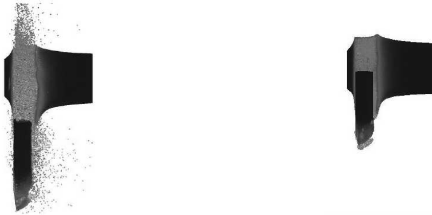
Figure 2.16: Screenshot for two simulations with stresses of the failed particles set to zero and failed particles converted respectively [50]
