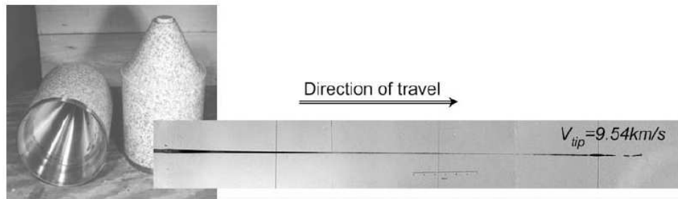
Figure 1.3: Copper liner and explosive on the left, flash X-ray of a jet in right [5]
