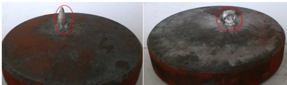
Figure 6.3: Sample image for 4th and 5th areal density targets (back face) in which the projectile was struck in the target and shattered after impact
