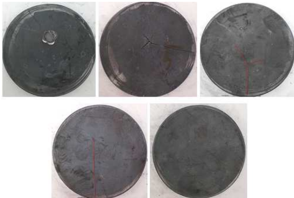
Figure 6.5: Post mortem images of the back faces of HRC 49.5 samples from the 1st to 5th areal density respectively
