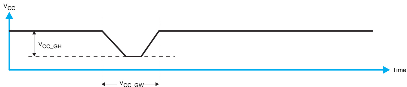
Figure 25. Glitch Width and Glitch Height
